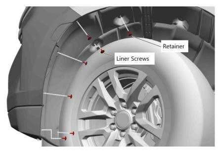
14. Pull back the wheelhouse liner. There will (3) front bumper fascia guide screws, loosen the top two bolts and remove the lower screw.
