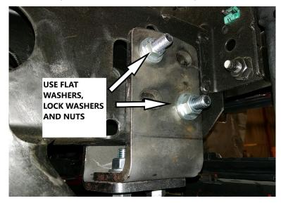
8. Mount the secondary bracket to the mounting bracket using 7/16" hardware.
