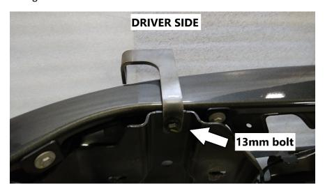
11. Set the top mounting brackets so that they are minimum of 36 ¾" and maximum of 36 7/8" apart.
