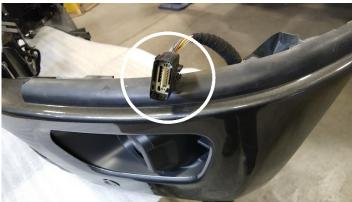
7. On models with sensors and/or adaptive cruise, you will need to unhook the connector from its location to remove the bumper.
