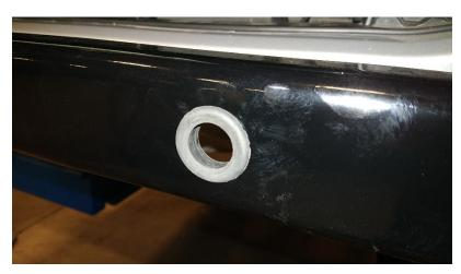
6. Insert sensors into the grommets. You may want to wipe a little WD-40 into the grommet opening to help insert the sensor. (DO NOT TWIST SENSOR).
