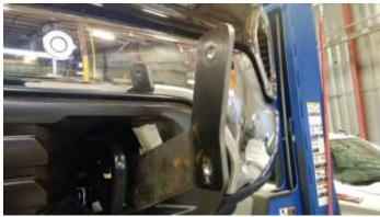
6. Reinstall the tow hooks. Use the factory tow hook bolts. If there are no tow hooks present, use ½" bolts. Also, at this time tighten the 18mm bolt that was loosened in step 1.
