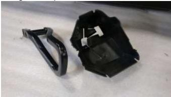
3. Also remove the tow hook trim panel. It is mounted by two 7mm screws and one clip.
