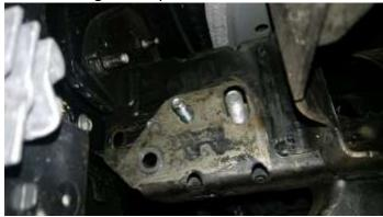
5. From the back side, slide the mounting bracket through tow hook opening. Use 3/8" and  $\frac{1}{2}$ " washers, lock washers and nuts to install.
