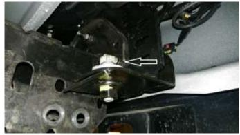
2. Remove the tow hook along with the plastic cover around it.
