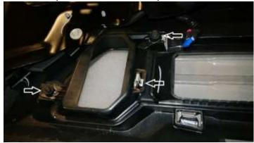
4. Slide the 5" tab w/the bolts through the top holes of the frame.
