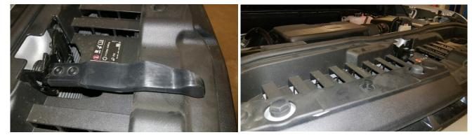
6. If vehicle is installed with a front camera, unhook the connector. The grille can then be removed by remove four 10mm bolts on top.
