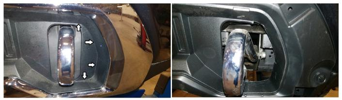
3. Remove the tow hook bolts and install the  $\frac{1}{2}$ " x 5" bolts. Mount the bottom bracket to the outside of the frame. Push the bracket upwards and tighten bolts and nuts.
