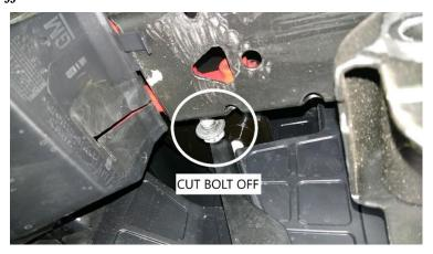
3. Remove the shield that is around the tow hook. There is a bolt on top and a clip on the bottom. You may have to cut it off.
