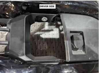
5. Before reinstalling the tow hooks, place the tab with the two bolts through the frame facing outwards. The ½" bolt will go through the large, slotted hole of the frame.
