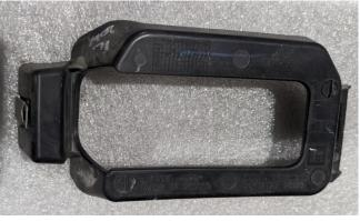
4. You will need to cut out the outside area of the tow hook opening. Measure 1/4" from the edge and use a utility knife to cut.
