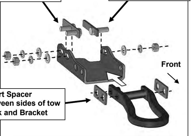
Insert Spacer between sides of tow hook and Bracket
