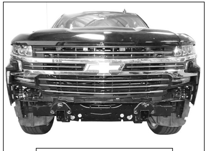
(Fig 8) Reinstall grille and cover
