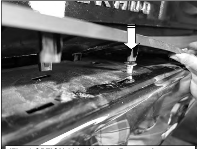
(Fig 5) OPTION 2014-16 only: Remove bumper bolts attaching bumper to inner bracket. Remove outer bumper first, then remove inner brackets
