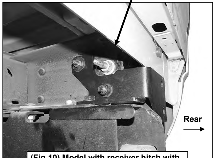
(Fig 10) Model with receiver hitch with support strap pictured (also see Fig 7)
