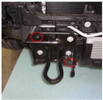
Figure 3a (TOW HOOK & OEM MOUNTING BRACKET)
