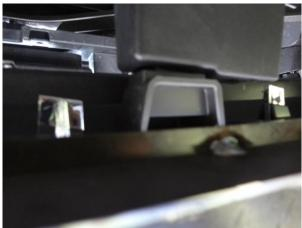
Figure 2c- example of clip holding grill
