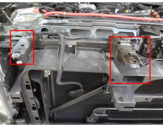
Figure 2a-bolts on LH side
