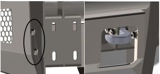
Figure 10a (bolt location for lower guard)
