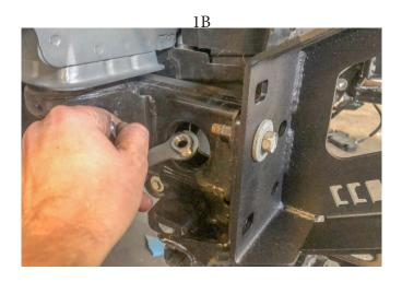
Slide in single nut retainer bracket into large hole in the back and tighten with bolt/washer as shown.
