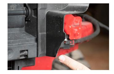
Using a flat head screwdriver or plastim trim removal tool, begin pushing the black grille frame away from the red cover.
