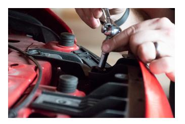
Shown right is a reference photo of the trimming required on the front area of vehicle once the grille is removed. This will need to be trimmed to allow proper fitting for the bumper.
