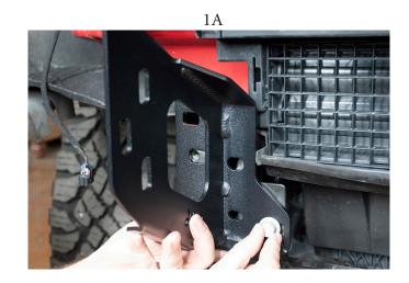
After hand tightening one of the stock bolts (See Fig 1B), you'll need to insert the provided bent nut retainer for the 2nd bolt to thread to (shown in Fig 1C/)
