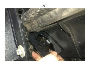
You'll then need to take the included bracket (2C) and place it on the inside of vehicle frame where the large bolt will go through (Fig 2A) and secured with washer and locking nut.
