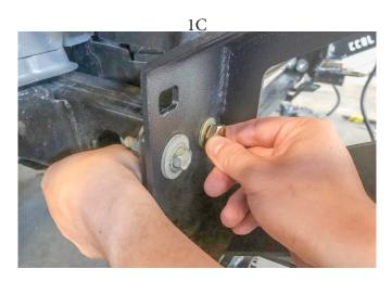
Next, you'll need to take the provided small back frame bracket and place it behind the large front braket and against the vehicle frame.
