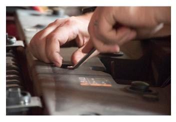
Remove bolts that are holding the top grille cover piece in place and pull off front grille.
