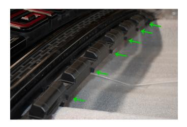
Shown to right is the "dog bone" 3 bolt piece that holds the bumper into place onto the frame bracket.
