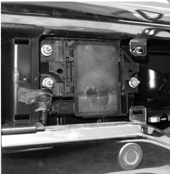
(Fig 13) Remove adaptive cruise control "ACC" and parking sensors (if equipped)
