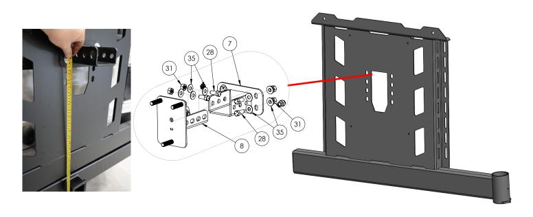
With the tire mounted, there could be a small gap between the back of the wheel and the Tire Mount Plate approximately 1/4"-1/2". This is ok because the tire is pressed against the Tire Carrier Back Plate. The tire should be tight against the back plate and not able to wiggle side to side or up and down. This keeps the tire from shaking on the tire carrier.
