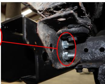
Install the 7/16" Hex Bolts, Washers and Frame Backing Plate as shown into the second set of holes in the rear Cross Member. You man need to lower the gas tank skid plate to access these holes to be able to insert the Frame Backing Plate behind the Cross Member. Leave these bolts loose while you finish the bumper installation.
