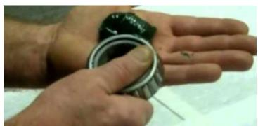
Next place the tire carrier Swing Arm upside down as shown in the image below. Insert the greased bottom bearing LM29749 into the housing with the tapered side facing into the housing.
