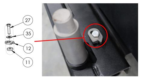
\*\*\*The Swing Stop is designed to allow the swing arm to rest in the open position when the Jeep is out of level. It is also a safety feature that will help stop the tire carrier Swing Arm from swinging around and damaging your Jeep. Repeatedly allowing the Swing Arm to swing around uncontrolled could damage the swing stop. Always open the Swing Arm and allow it to gently rest against the Swing Stop.\*\*\*
