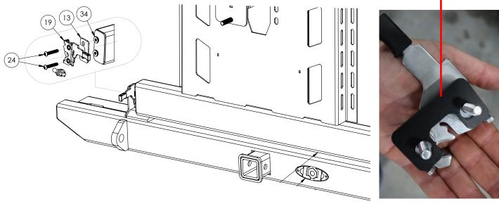
Next install the Striker Bolt with Yellow Zinc plated Washers and Metric M10 Nut. Just snug these up for now until all adjustments are made. Also install the small rubber bumper as shown.
