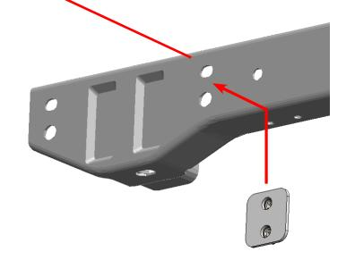
Install the Bottom Bracket as shown using 3/8" Hex Bolt and washers into the bumper. You will need to use the existing leaf spring mounting bolt to install the bracket to the frame.
