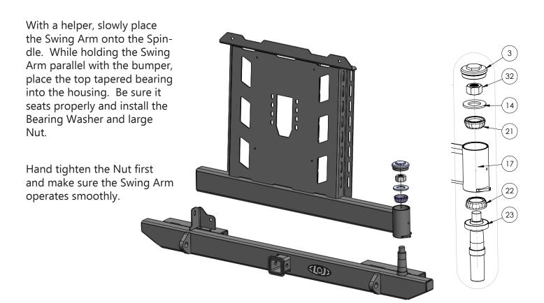
It is a good idea to add a little blue loctite to the Nut to prevent loosening. Slowly tighten the nut using a 1-1/2" Socket. Check the swing arm movement every 1/8th turn. The Swing Arm movement should not be restricted and should move freely. Overtightening could damage the bearings.
