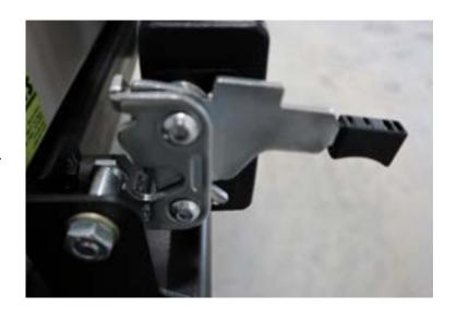
Always close the tire carrier Swing Arm by pushing on the arm near the Latch or the bottom of the tire. This helps to insure the Latch catches the Striker Bolt securely.
