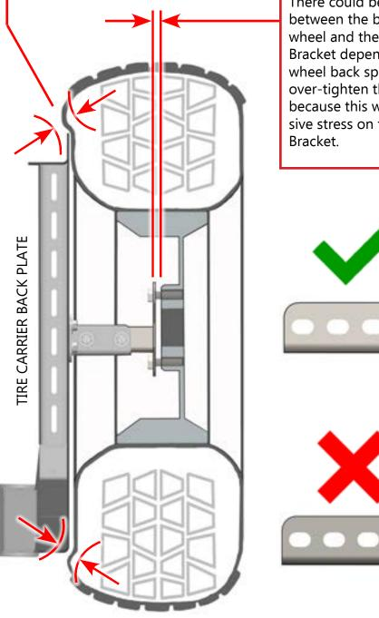
There could be a small gap between the back face of the wheel and the Tire Mount Bracket depending on your wheel back spacing. Do not over-tighten the lug nuts because this will cause excessive stress on the Tire Mount Bracket
