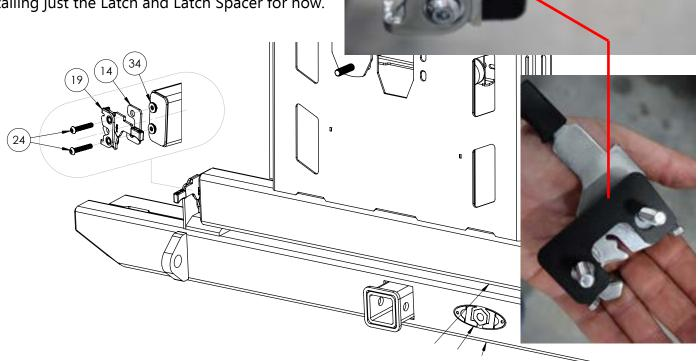
Next install the Striker Bolt with Yellow Zinc plated Washers and Metric M10 Nut. Just snug these up for now until all adjustments are made. Also install the small rubber bumper as shown.
