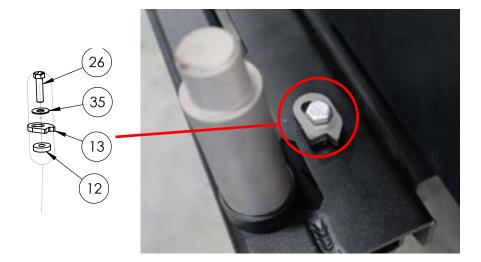
\*\*\*The Swing Stop is designed to allow the swing arm to rest in the open position when the Jeep is out of level. It is also a safety feature that will help stop the tire carrier Swing Arm from swinging around and damaging your Jeep. Repeatedly allowing the Swing Arm to swing around uncontrolled could damage the swing stop. Always open the Swing Arm and allow it to gently rest against the Swing Stop.\*\*\*
