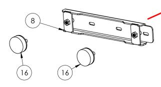
Install the Bumper Door Bracket so the two large bumpers line up with the ribs on the back of the tire carrier Swing Arm. Adjust the Bumper Door Bracket as needed and tighten securely.
