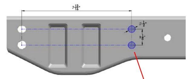
To improve your drilling accuracy it is a good idea to start small bit and get progressively larger or use a step drill. Be careful when you punch thru as to not hit the gas tank behind the cross member.
