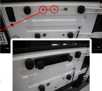
Install the Tire Mount and Tire Mount Bracket onto the Swing Arm using 7/16" Hex Bolts, Nuts and Washers. You will want to mount this in the lowest position that will work for your size tire. Measure the radius of your tire then transfer that measurement up from the top of the bumper to find the optimal position for your Tire Mount.
