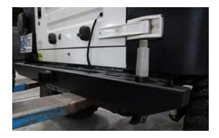
Install the 7/16" Hex Bolts, Nuts and Washers into the two outside mounting holes first. Leave these slightly loose while you finish the bumper installation
