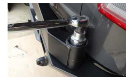
Install the tire carrier Swing Stop. Be sure to adjust it to allow the Swing Arm to open completely and allow full use of your tailgate and tighten securly. If you have accessories mounted on your tire carrier, you can adjust this slightly to help avoid the accessories hitting the Jeep when you open the Swing Arm.
