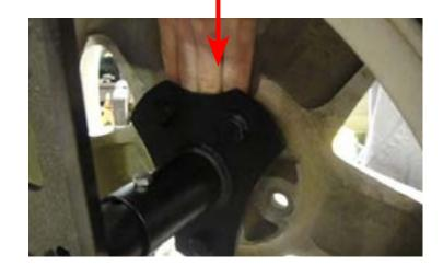
Your tire should squeeze againse the back plate of the tire carrier at the top and the bottom.
