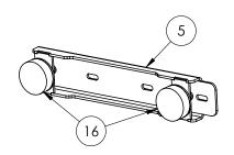
Install the Bumper Door Bracket so the two large bumpers should line up with the ribs on the back of the tire carrier Swing Arm. Adjust the Bumper Door Bracket as needed and tighten securely.
