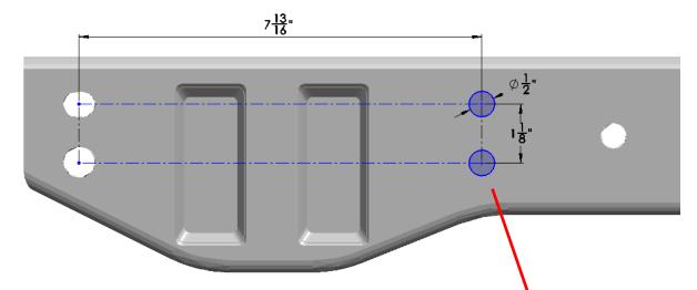
To improve your drilling accuracy it is a good idea to start small bit and get progressively larger or use a step drill. Be careful when you punch thru as to not hit the gas tank behind the cross member.
