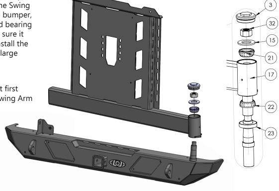
It is a good idea to add a little blue loctite to the Nut to prevent loosening. Slowly tighten the nut using a 1-1/2" Socket. Check the swing arm movement every 1/8th turn. The Swing Arm movement should not be restricted and should move freely. Overtightening could damage the bearings.
