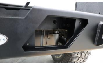
Install the 7/16" Hex Bolts, Washers and Frame Backing Plate as shown into the holes that you drilled into the rear Cross Member. With the gas tank skid plate lowered as shown, you will be able to insert the Frame Backing Plate behind the Cross Member. You can access bolt holes thru the light bezel opening in your bumper.
