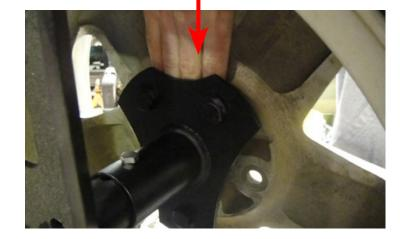
Your tire should squeeze againse the back plane of the tire carrier at the top and the bottom.
