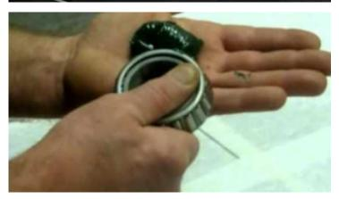
Next place the tire carrier Swing Arm upside down as shown in the image below. Insert the greased bottom bearing LM29749 into the housing with the tapered side facing into the housing.
