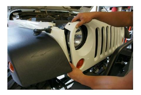
ONCE LOOSE, THE ENTIRE PLASTIC SCREW AND EXPANSION SLEEVE SHOULD PULL UP AND OUT OF THEIR MOUNTING HOLES.
