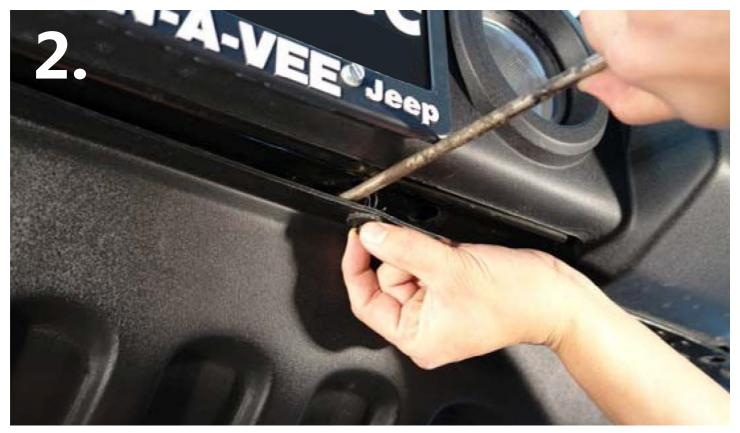
Once unscrewed, you should be able to pull out both the plastic screws and insert with little effort but if you find the screws just spin, you will need to wedge a flathead screwdriver between your JK's plastic bumper and air dam to help you remove it.
