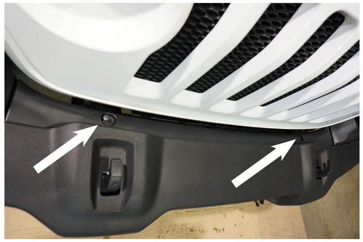
You can now remove the trim strip (2 vertical clips, 4 horizontal, 2 screws) to access the bumper mount bolts.
