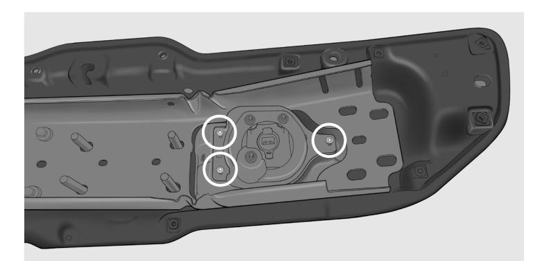
Once the plastic trim piece is off, remove the three T-20 screws (circled) that hold the foglight housing in place. The next step will show you how to remove the light from the housing.
