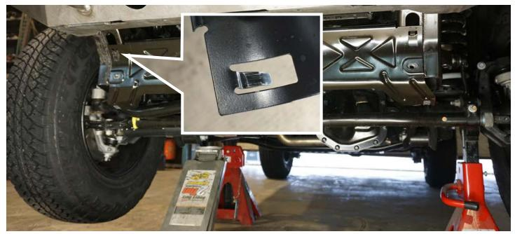
Also remove the crash bar, there are two bolts holding it on.
