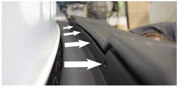
You can now remove the trim strip (2 vertical clips, 4 horizontal, 2 screws) to access the bumper mount bolts.
