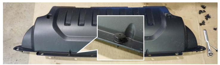
The skidplate is held to the vehicle with eight (8) clips in the front, and the two bolts you just removed, on the bottom.
