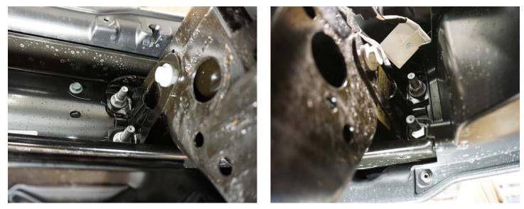
The bumper is secured to the vehicle with four (4) bolts on both sides. Remove these and the bumper should come of the vehicle.
