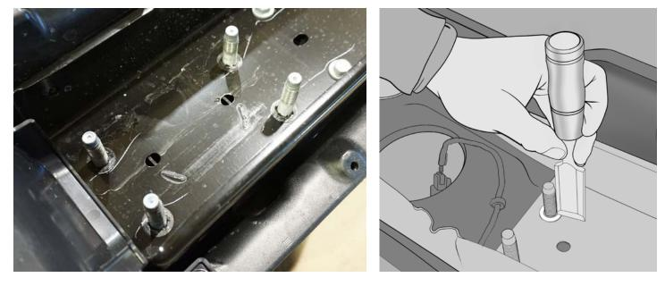
The bolts that hold the bumper together are held in place using locking tooth washers, you can either pry them up with a screwdriver, or cut them off using a sharp chisel or similar tool.
