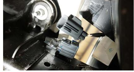
Undo the harness plug that connects the foglights to the vehicle.
