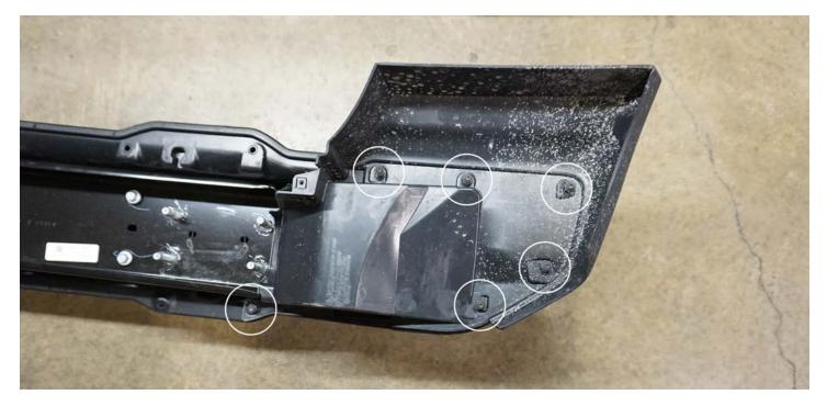
Next, remove the labeled T-25 screws from the bumper, this will allow you to access the foglight, located underneath.
