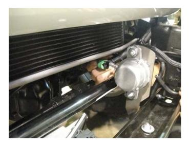
**8a.** Connect the vacuum lines that were removed earlier.
