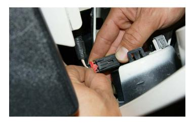
**26.** Squeeze the wiring harness plug and pull it out of your Jeep JK Wrangler's indicator light socket. You can now pull the grille off and set it aside for now.
