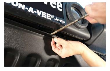
**3.** Now, climb under the front of your Jeep JK Wrangler and using a phillips screwdriver, remove the remaining 2 plastic screws securing the air dam to the lower cross member. As before, if these screws just spin in place, use a flathead screwdriver or small pry bar to help you force them out.
