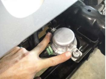
**4a.** With the switch out of the way cut the tab off that is closest to the front of the Jeep as shown in the photo.
