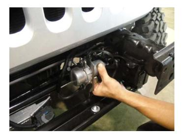
**7a.** Bolt the switch into place on the bracket.
