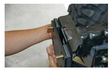
**16.** With the help of a friend, carefully place your new LoD Signature Series JK Front Shorty Winch Bumper on to the frame rails of your Jeep JK Wrangler and slide the mounting holes through the bolts you just installed. Reaching from the back, loosely secure it in place using the nuts provided.
