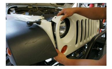
**25.** Lean your Jeep JK Wrangler's grille forward a bit to gain access to the indicator lights. Then, take the wiring harness plug and pull the red locking tab back.
