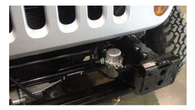
**2a.** Begin by removing the green clip that secures the vacuum line to the switch. Simply slide the clip down and pull the line off the switch.
