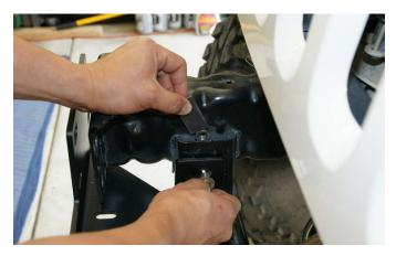
14. Slide one of the steel spacers in between the LoD Signature Series winch plate and frame rail bumper mount on your Jeep JK Wrangler. Then, insert the long bolts and washers provided with the bumper through the mounting holes and spacer as shown in this pic.
