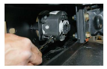
**23.** Using a phillips screwdriver, loosen the plastic retaining screws securing the top of your grille to your Jeep JK Wrangler.
