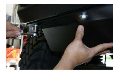
**33.** Secure the LoD Signature Series skid plate to the lower cross member of your Jeep JK Wrangler using the bolts and washers provided. You will need a 9/16" socket and wrench for this job.
