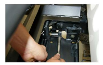
**18.** Accessing the bolts and nuts through the fog light holes on your LoD Signature Series JK Front Shorty Winch Bumper, tighten up the (4) mounting bolts and nuts located on the outside of your Jeep JK Wrangler's frame rails using a 3/4" socket and wrench.
