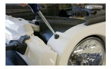
**24.** Once loose, the entire plastic screw and expansion sleeve should pull up and out of their mounting holes.
