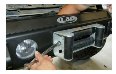
**29.** Carefully place your winch on top of the LoD Signature Series winch plate and then reinstall your Jeep JK Wrangler's grille as shown in this pic.
