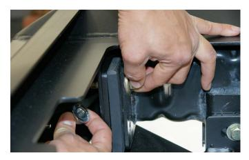
**17.** Using a 3/4" socket and wrench, tighten up the (4) mounting bolts and nuts on the inside of your Jeep JK Wrangler's frame rails as shown in this pic.
