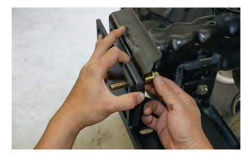
**15.** Repeat step #14 until all the steel spacers are installed in between the LoD Signature Series winch plate and frame rail bumper mount and that all the bolts are sticking through them as shown in this pic.
