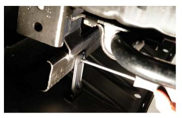
**4.** If your Jeep JK Wrangler came equipped with factory fog lights, climb under the front of your Jeep, look up behind the front bumper, locate the wiring harness plug, lift up the clip and then pull it off as shown in this photo.
