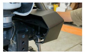
**19.** Using a 3/4" socket, tighten up the LoD Signature Series winch plate frame rail mounts as shown in this pic.
