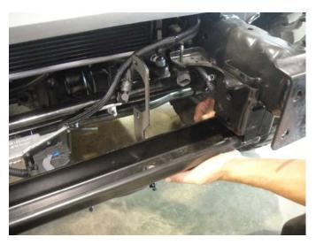
**6a.** With the bracket installed bolt the vacuum switch to the bracket as shown. The switch will be repositioned on its side in the new bracket.
