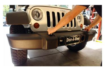
**10.** Using a phillips screwdriver, remove the 2 plastic screws securing the top plastic cover in place.
