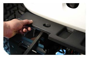
**12**. Again, if your Jeep JK Wrangler came equipped with factory fog lights, use a phillips screwdriver to remove the 4 screws securing them to the bumper. Then, pull the fog lights out and set them aside until you are ready to install them in your new LoD Signature Series JK Front Shorty Winch Bumper.
