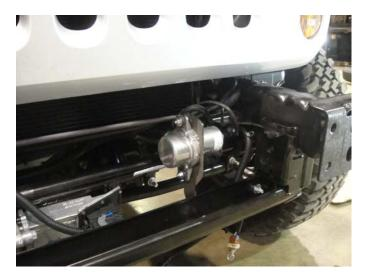
**9a.** When finished the vacuum switch should look like the pic to the right.
