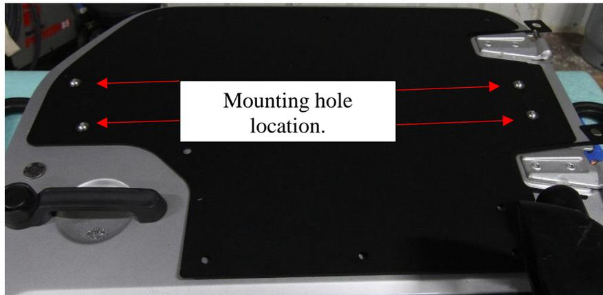
6. Next with the door skin secured to the door, center punch the remaining mounting holes. Make sure the door skin is pressed flush to door before center punching the mounting hole.
