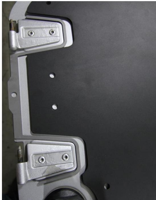
2. Once you get the door skin into desired location, using a transfer punch center punch the four mount holes located in the center of the door skin.
