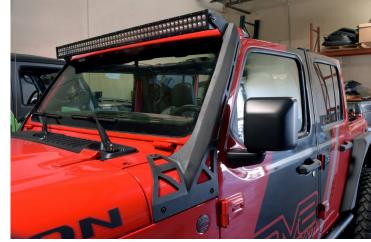
Optional: Prior to installation, you can use single sided sticky foam  $(\frac{1}{4})$  to cushion between the bracket and the Jeep.
