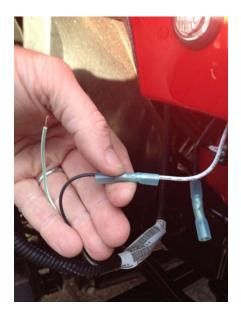
5) Install butt connectors. The LED's are polarity sensitive (will only light with power going one way). This 2014 JK needed wires to be black/white and white/black for the LED's to illuminate. Use a lighter to shrink the butt connectors covers. Tuck wires away, and you are complete.
