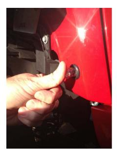
4) Make sure marker light power is off, and cut the two wires that fed the factory marker lights on OEM plastic fenders.
