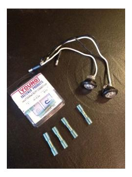
1) Install butt connectors on LED's
