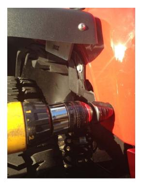
3) Slide grommet off plastic portion of LED. Slide into the 3/4" hole. Push grommet through hole and set it. Then push LED into grommet.
