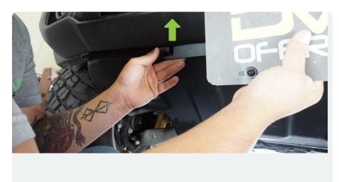
STEP 4 | When the bracket is pushed up into place, slide it to the driverside and then pull it down to seat it into place.
