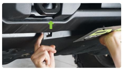
**STEP 5** When the bracket is pushed up into place, slide it to the driverside and then pull it down to seat it into place.
