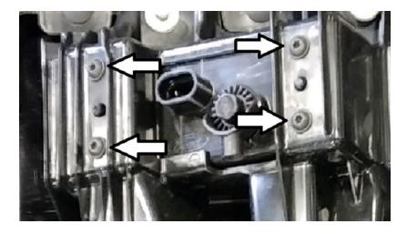
3. Mount the fog light to the fog light bracket by reusing the factory Torx screws. The brackets are driver/passenger specific.
