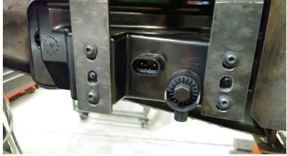
4. Mount the bracket with the foglight attached onto the bumper using the included 5/16" hardware.
