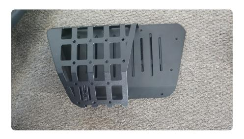
**STEP 7** | Mark the mounting holes using a sharpie, and do not let the pocket and panel shift.
