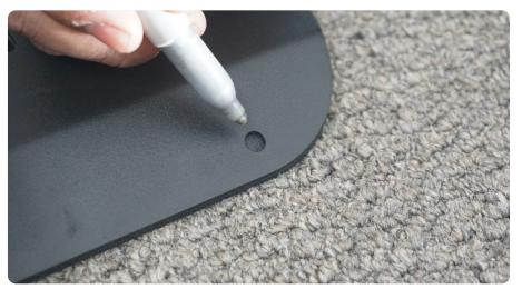
**STEP 8** | Remove the pocket, and using a 17/64" drill bit, carefully drill the marked mounting holes.
