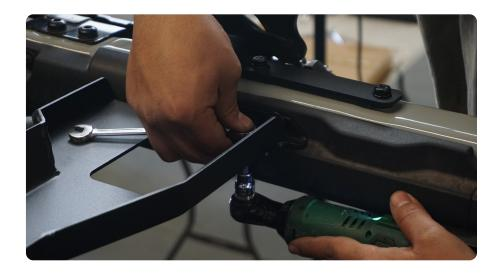
STEP 16 | Use an 8mm wrench to secure the factory hardware holding the roll bar bracket to the roll bar.
