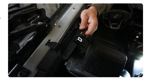
Loosely install the pressure plate.
