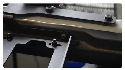
STEP 17 | Use a 13mm socket or T50 torx bit to secure the hardware holding the mounting plate to the rollbar.
