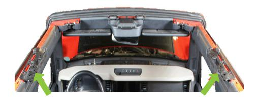
STEP 11 | Use a 8mm wrench to remove the bolt on the interior of the roll bar.
