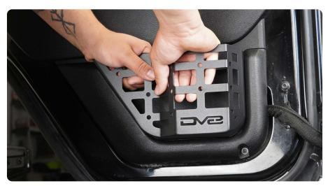
STEP 5 | Put the provide spacer, hardware, flat washer a mounting tab together as shown.
