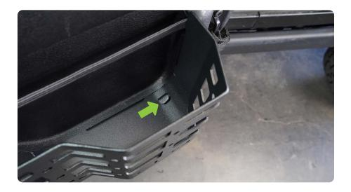
STEP 7 | While pressing down on the pocket use a phillips head screw driver to secure the Molle Pocket in place.
