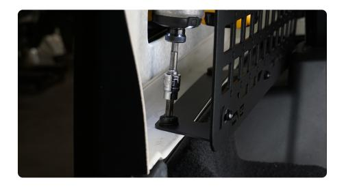
Secure all M6 hardware with 4mm allen bit and 10mm wrench.
