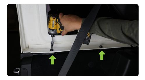
STEP 6 | Maneuver the panel into the approximate location of install and very loosely secure it with the factory hardtop bolts by hand.
