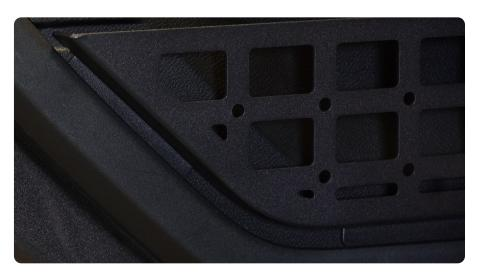
STEP 4 Using a T15 Torx Bit, remove the (2) factory door pocket screws and set aside.
