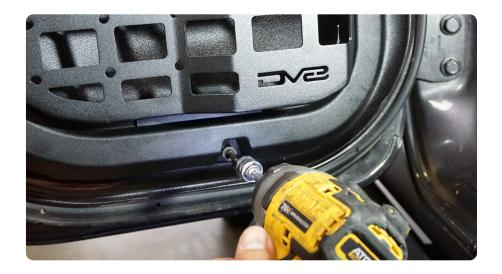
STEP 5 Using the provide hold down bracket and factory hardware, secure the DV8 Molle Pocket in place.
