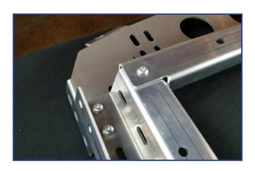
Attach rear reinforcement brace to front internal fascia frame as shown with 5/16" bolts. Repeat on both sides and keep bolts loose.
