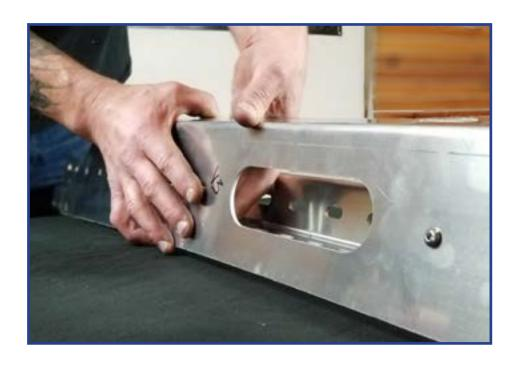
Shallow angle faces towards front end of roof rack as shown below
