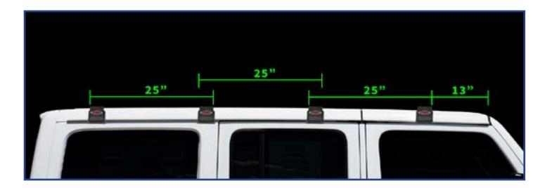
As a final rough check of your rear most gutter mounts, it should roughly have around 5 3/4" to 6" of space from the left side of gutter mount to the end of the rear gutter.
