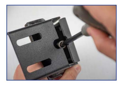
Once all your gutter mounts are prepped, you can now place them on the gutter and tightened a little but still be able to slide them side to side. (4 gutter mounts per side)
