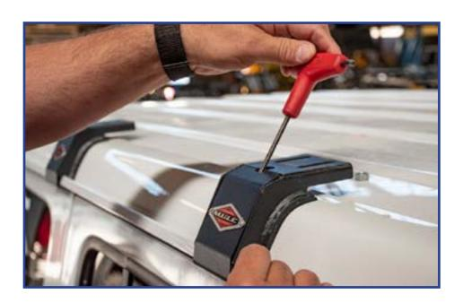
Pictured below are the dimensions you'll need to adjust your gutter mounts to. Starting from the front of vehicle where the gutter trim starts, measure out to 13" and place the right edge of gutter mount to the 13" mark. Once in place, go ahead and tighten it down.
