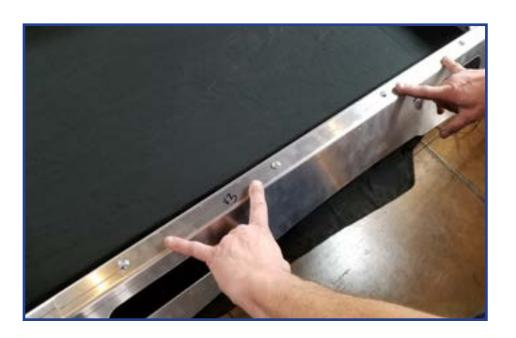
Next attach rear corner connectors with 5/16" bolts shown in photo below. (remember to hand tighten but keep fairly loose!)
