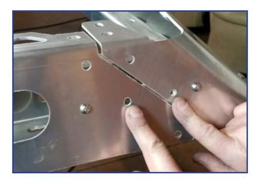
Attach front fascia piece shown bottom left photo along with a single spacer piece for each hole.
