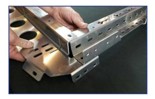
ATTENTION: When assembling the Mule Ultra Rack, remember to hand-tighten all bolts relatively loose until the very end of the install. This allows everything to fit into place before everything is tightened down.
