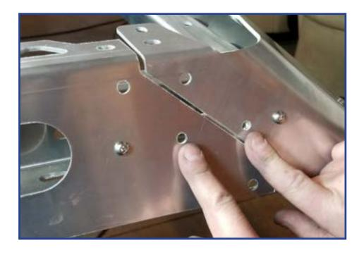
Next, attach reinforcement spacers as shown on all 6 hole locations with provided bolts & nuts. There are three mounting hole locations on each side.
