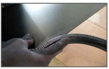
Install the weather stripping to the bottom of front fascia as shown and trim any excess.
