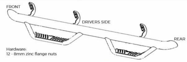
Identify the driver and passenger bars. The center bracket is closer to the front of the truck.
