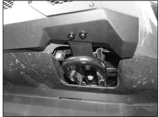
(Fig 20) Driver/left Support Bracket attached to inside of Bumper (model with tow hook)
