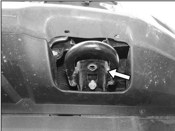
(Fig 9) Models with tow hooks, remove forward bolt and loosen but do not remove rear bolt to hold factory double nut plate in place in frame
