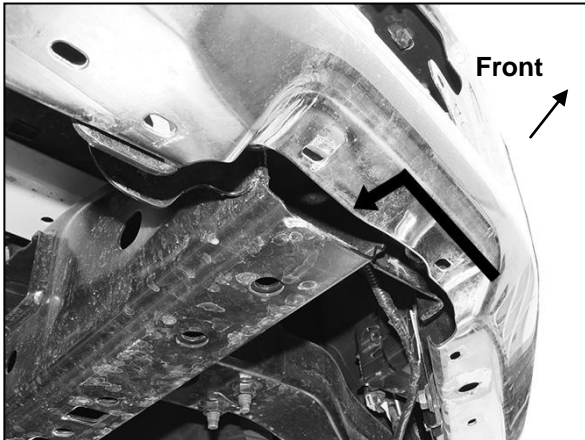
(Fig 11) Models without tow hooks, remove bottom hex nuts attaching bumper to bracket (Fig 4). Loosen the front hex nuts and tilt the bottom of the bumper out enough to insert the Double Nut Plates into the end of the frame (arrow).
