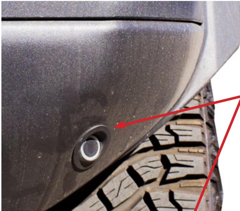
**Sensor bezels should be pointed up like OEM does**
