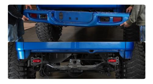
STEP 12 | If equipped with factory bed slider mounts, use a 16mm and 18mm socket the remove the bolts securing the mounting brackets.
