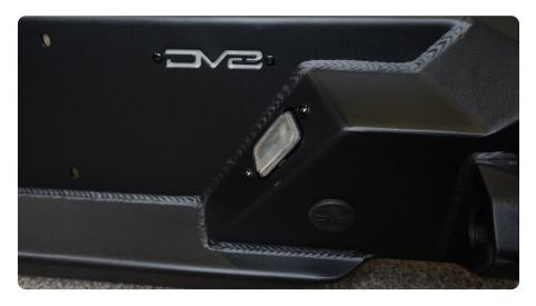
STEP 19 | Install the wiring connectors to each license plate light by pressing them into place.
