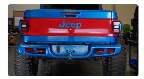
STEP 10 | Using the 16mm socket, remove the four bolts ((2) on each side), holding the bumper to the hitch.
