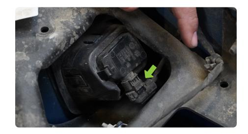
STEP 16 | There are four tabs on the outside of the license plate light. Three of four need to be lifted for light to be removed.
