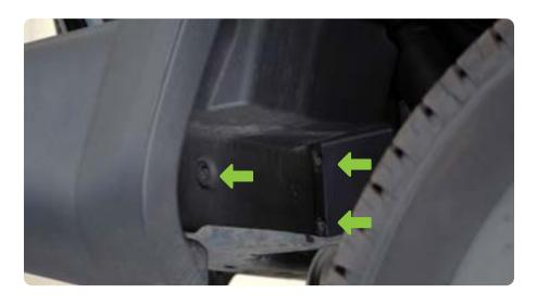
**STEP 4** Use a 16mm socket to remove the bolts securing the bumper brackets to the bumper. These are located on the edges of the bumper behind the rear tires.
