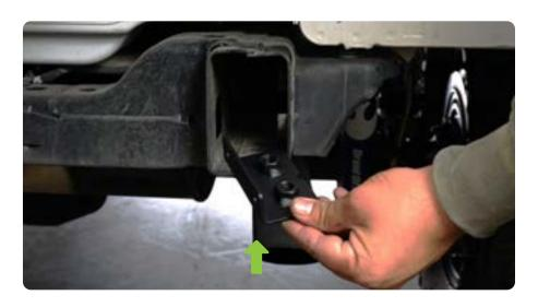
**STEP 9** I Install the flat nuts into the top two mounting holes on each side of the bumper by pressing them into place.
