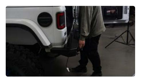
STEP 20 | Align the bumper left-toright and up-and-down. Check the wings to ensure neither are touching the body of the vehicle.
