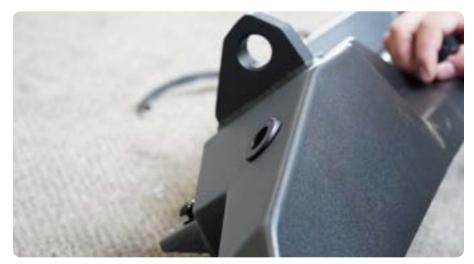
**STEP 12** With the bezels in place, run the sensor wiring harness though cavity in the bumper aligning the sensors with the bezels. Push Sensors into bezels ensure they have "clicked" into place. Secure sensor harness using provided zip tie tabs.
