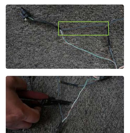
**STEP 14** | Using wire cutters, cut the wire and prepare ends for wire connectors.
