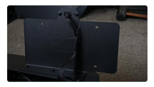
STEP 17 | Place the provided nut plate into the passenger side of the frame with the nuts facing upwards.
