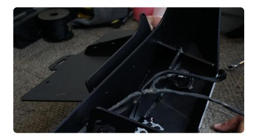
STEP 15 | Install the provided foam onto the license plate light.
