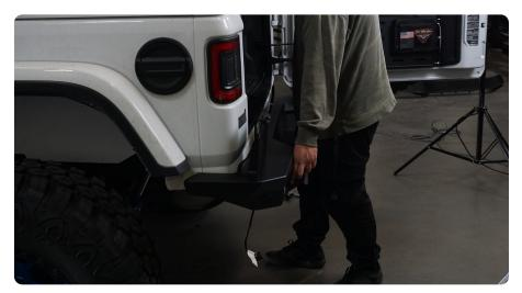
STEP 21 | Using a 18 and 21mm socket, ensure bottom bolts are tight enough to take the weight of the bumper.
