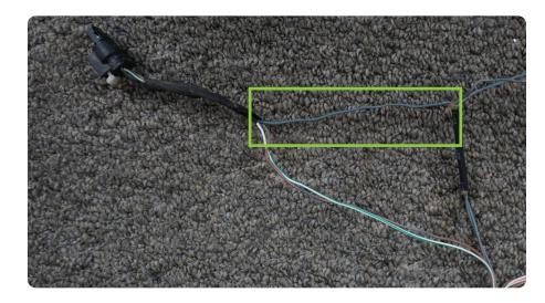
$\begin{array}{c|c} \text{STEP 11} & \text{Using wire cutters, cut the} \\ \text{wire and prepare ends for wire connectors.} \end{array}$
