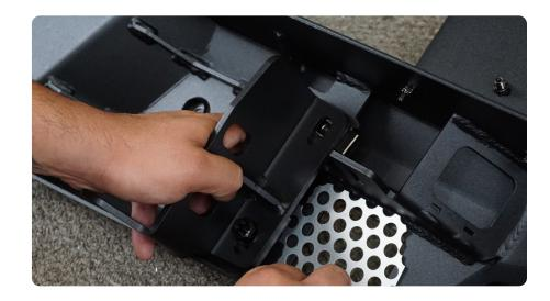
STEP 20 | With the mounts installed, lift the bumper onto the Jeep. Using the factory hardware on the driver side, and the provided M12 bolts on the passenger, loosely mount the bumper to the vehicle.
