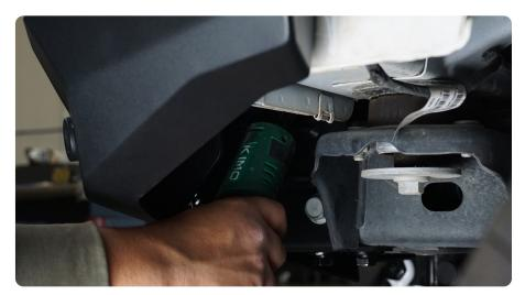
STEP 22 | Adjust the in-and-out position of the bumper ensuring there are consistent gaps between the bumper and vehicle, and that the bumper is not touching the vehicle.
