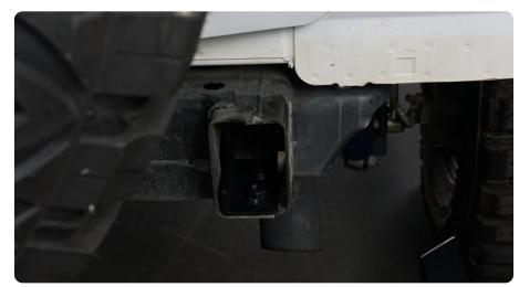
$\begin{array}{c|c} \text{STEP 18} & | & \text{Install the clamp nuts} \\ \text{onto the bumper.} \end{array}$
