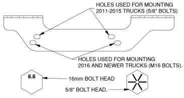
Figure A3: Passenger side plate and bolt head configurations. PAGE 2 of 5
