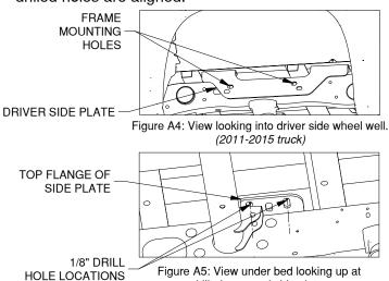
**4. Enlarge the holes.** Use the 1/8" holes as pilots, drill out each hole with a 9/16" bit.
