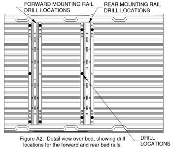
The fuel tank of the truck may be directly below the area of the bed which needs to be drilled. Always carefully examine the area under the truck where drilling will occur before drilling. Make certain that the tank, or other equipment, is not damaged during drilling. Damage to the tank may result in property damage, serious injury or death.
