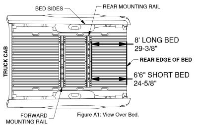
**IMPORTANT:** The mounting rail is designed to install only at the described location. Failure to place the mounting rail precisely may result in added difficulty during installation and/or property damage.
