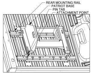
Figure C3: View into truckbed looking towards tailgate.
