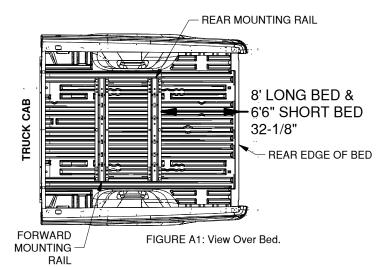
**IMPORTANT:** The mounting rail is designed to install only at the described location. Failure to place the mounting rail precisely may result in added difficulty during installation and/or property damage.
