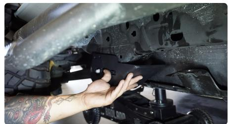
STEP 16 | Have a friend hold the plate into place or use a jack/stand to keep the two upper mounting holes aligned.
