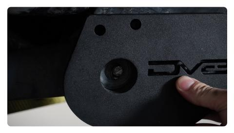
STEP 15 | Swing the plate up to hug the frame rails, and push the bolt back through slightly, allowing the skid to hang from the bolt.
