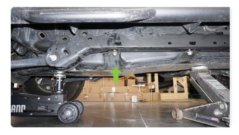
STEP 3 Use an 18mm socket to remove the (3) bolts along the passenger frame rail, and the (2) bolts securing the skid to the front cross member.
