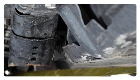
STEP 9 Drill the two mounting holes out using a 25/64" drill bit.
