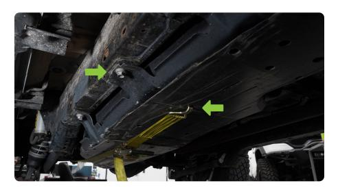
STEP 11 | Jack the vehicle off the ground slightly using a floor jack.
