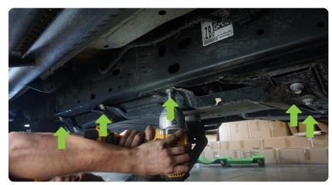
STEP 4 Use an 18mm socket to remove the bolt securing the gas tank skid located **under** the rear driveshaft.
