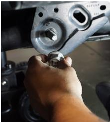
STEP 13 | When the ratchet strap is tensioned correctly, the bolt should slide out and back in fairly easily with a few decent hits with a rubber mallet.
