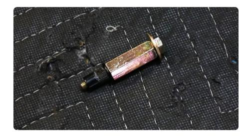
$\begin{array}{c|c} \text{STEP 12} & \text{Slide the nutsert tool with} \\ \text{the nutsert into the mounting hole.} \end{array}$
