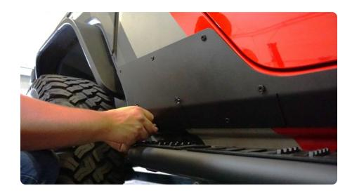
STEP 9 | Secure the M5 hardware using a #3 allen bit.
