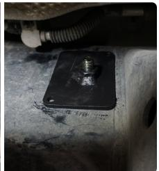
STEP 3 | Loosely attach the slider rails center mount to the frame using the provide M12x105 hex bolts using a 18mm wrench.
