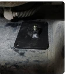
STEP 10 | Loosely secure the slider rail center mount to the frame using provided M12x120 hex bolts, square nut plate and 18mm wrench.
