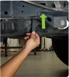
STEP 5 | Loosely secure the rear slider mount using a M12x105 hex bolt into the nut plate with handle using a 18mm wrench.
