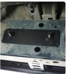
STEP 11 | Loosely secure the rear slider rail mount to the frame using a M12x120 hex bolt, square nut plate and 18mm wrench.
