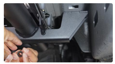
STEP 4 | Once all hardware is loosely installed, secure the DV8 OE Steps in place using a 13mm socket.
