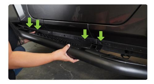
STEP 3 | Loosely secure the steps with the provided M8 hardware.
