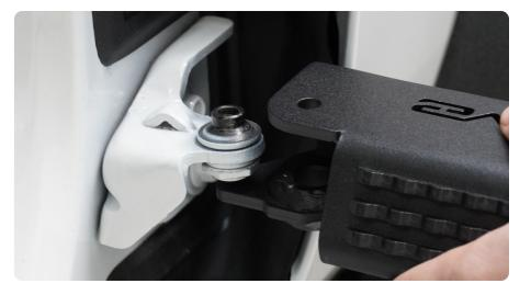
**STEP 4** | Slip the foot peg into place and loosely secure with the provided M8 hardware.
