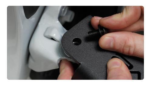
**STEP 5** | Hold the foot peg in the desired position and tighten the M8 hardware with a #5 allen bit.
