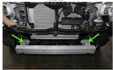
You will also need to remove the aluminum reinforcement frame or sub-bumper shown in Fig 4C.
