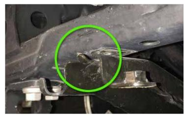
With the help of a friend, place the bumper onto the frame brackets and check for alignment around the front end. If spacing is fairly even from the bumper to the body of vehicle, go ahead and secure the front bumper to the frame brackets with provided hardware.
