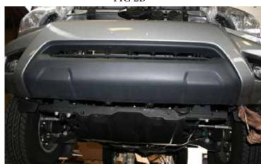
For this step, you'll need to carefully unclip and slide the trim piece towards you so as not to break the tab that secures this into place for later. (Fig 2C / 2D)
