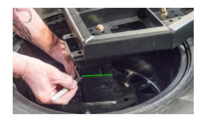
Flip arm over and position your tire mount into position. Tighten into place 1/4" past where you marked your lines.
