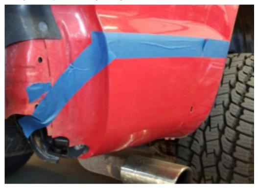
We will also need to remove some of the plastic clips inside the fender well to pull away the inner fender flap so we don't cut into it.
