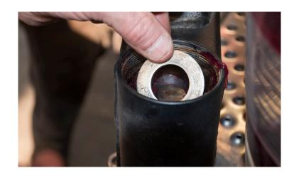
Drop your large bolt into place and tighten down into place till its nice and tight. Then nudge it back a hair so it won't bind.
