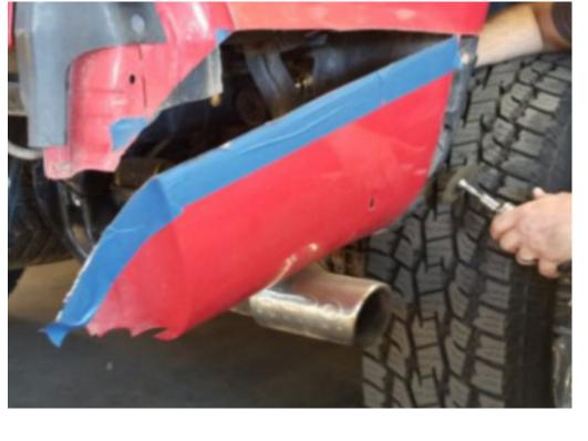
We will also need to remove this reinforcement piece inside each fender well
