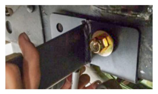
On the other end of the bracket (shown below) we'll need to secure that to the bumper that wraps around the side of vehicle. Secure these with the included 3/8" bolts, nuts and washers.
