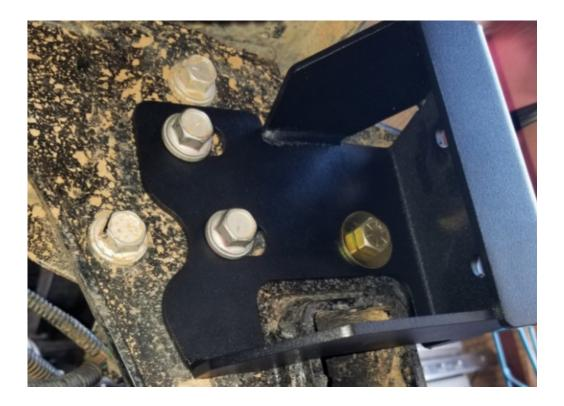
We're now ready to place the bumper onto the frame brackets. From here, you'll use 1/2" bolts, washers and nuts on each side to secure bumper into place. You can tighten down these bolts once you are happy with proper spacing all around. Go ahead and tighten down the internal frame bracket bolts as well. (pictured above)
