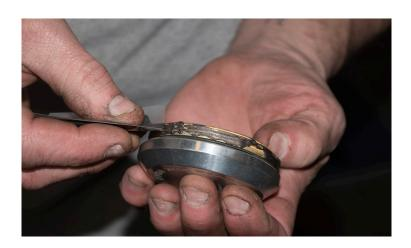
Attach cap onto spindle and tighten down. You may need to twist counter clockwise while applying pressure until you hear a click -- then tightn down clockwise.
