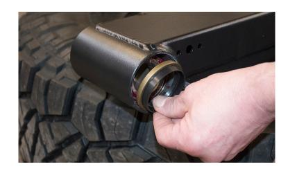
Place arm into position, holding the bearing/grease seal with hands, onto the spindle.
