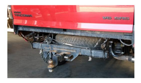
Next, we'll take the frame reinforcement brackets starting with the driver's side and attach to the frame of vehicle. You'll be re-using two stock frame bolts you removed to take stock bumper off and (1) provided 1/2" bolt, nut and washer.
