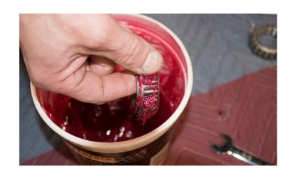
Place your greased bearing ito the bottom of the arm as shown.
