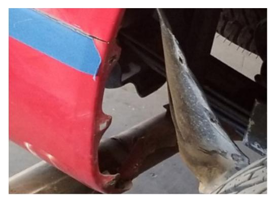
We can now begin cutting the lower portion of the bumper off. Carefully follow the top of the masking tape.
