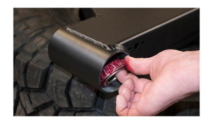
Now place grease seal as shown inside the bottom of the arm.
