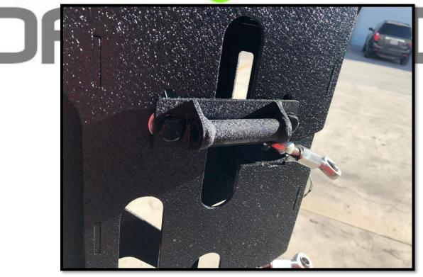
10. Install heims onto carrier door. With the door closed and parallel with the rear hatch plate, adjust heims so that they line up with tabs on rear hatch plate.
