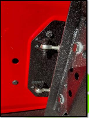
11. Once installed, if there is any play on the carrier when the hatch is closed, either the heims need to be adjusted inwards, or you can space the stopper on the carrier arm with one or two washers so there is a firm fitment when closed.
