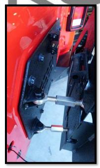
12. Remove factory third brake light from stock carrier. Attach to new carrier using (4) factory screws.
