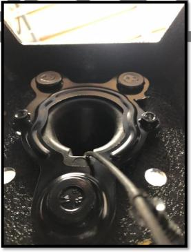
18. Using the provided camera enclosure, cover the camera and bolt using supplied flush mount allen head bolts.
