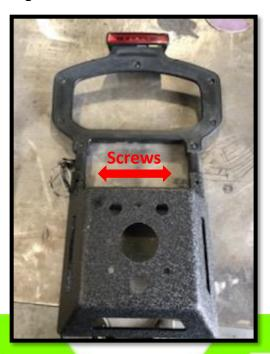
13. If you are running a rear camera you will utilize the factory camera bracket (plastic) and the provided camera enclosure. If you do not have a camera, you will utilize the block off plate.
