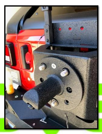
19. Place spare on carrier. Open and close carrier to sure all parts are moving properly.
