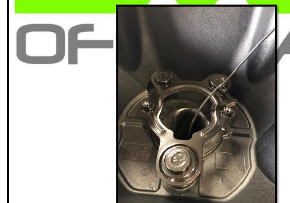
16. Using a punch, lightly tap out the factory camera mount. NOTE: This is plastic and so be careful and punch out the two holes in the center equally.
