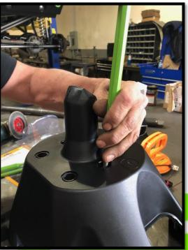
17. If using a camera, place the factory camera mount (plastic) though the holes. Place the factory stud plate behind it. Secure using factory bolts.
