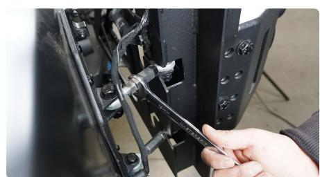
$\begin{array}{c|c} \text{STEP 30} & \text{Check and adjust the tire} \\ \text{catch up/down so that the stopper lands} \\ \text{in it when the tailgate is closed.} \end{array}$
