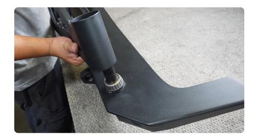
STEP 15 | Then install the race and remaining bearing as shown with the race being placed first, and the bearing on top, facing down.
