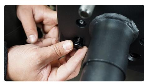
STEP 27 | Adjust the camera tube and secure using the provided M6 hardware with a #4 allen bit.
