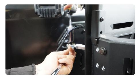
STEP 29 | Adjust the heim joints by turning the center connector nut.
