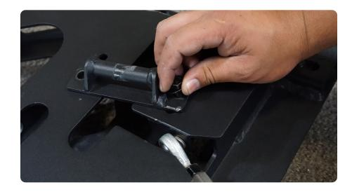
STEP 12 | Install the carrier "catch" using the provided M8x45 hardware.
