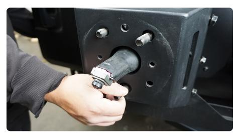
STEP 24 | Secure the factory rear camera/ tire mount to the DV8 Tire Carrier using the (2) factory torx head screws previously removed.
