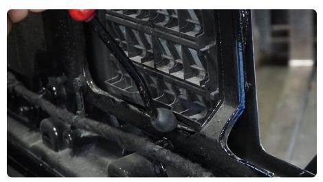
STEP 8 Using a dremmel or cutting tool of choice, remove the three sided border from the fin vents.
