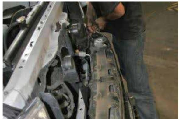
Remove the large metal bracket extending across the bumper with a 10mm socket and/or wrench.
