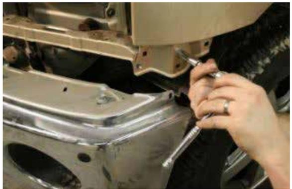
Now unbolt the chrome outer shell of the bumper to expose the aluminum bumper underneath.
