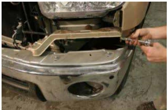
Remove the bumper attached to the frame rails. Next remove the outer aluminum curved piece (shown at right) and then remove the bracket behind it. Both pieces need to come off.
