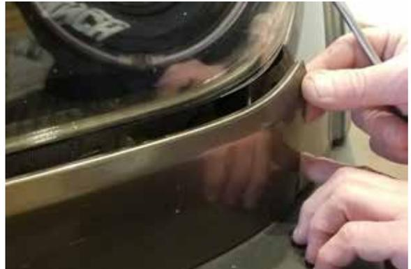
The best we have found to remove the panel is to use a flat head screw driver covered with a piece of tape (to protect the paint). Slide in the screwdriver and carefully rotate it to release the plastic clips. \*\*If these panels are removed at the wrong angle there is a molded piece that will break off so use caution.
