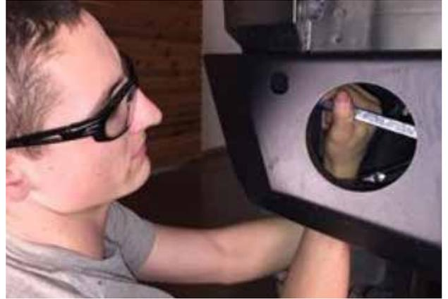
In the center step of the bumper there are 2 holes for 1/2" button head bolts. These bolt locations are mainly used for the optional winch mount and are not required for regular use; however, if you desire to install the bolts we recommend using the additional USS flat washers as shims between the bumper and the factory receiver hitch assembly.
