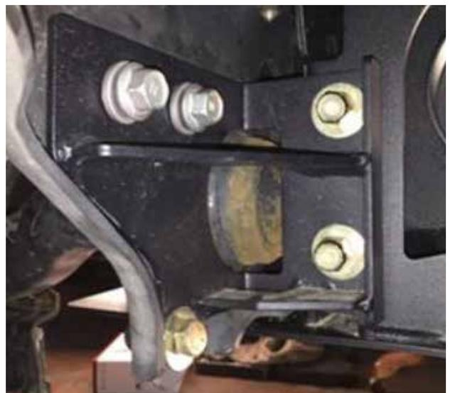
Adjust the bumper as desired, then tighten all bolts. We recommend tightening the top 2 socket cap bolts utilizing a hex key first.. this will help the bumper from shifting as you tighten the rest of the bolts. It is also recommended you tighten the oem bolts on the mounting brackets last.
