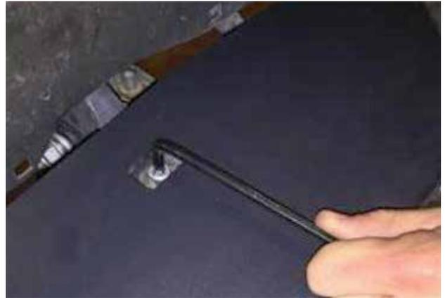
Install the 3/8" hex cap bolt with corresponding washers and nyloc (again using washers on both the nut and bolt sides), in the holes previously drilled out. Again keep all nuts and bolts loose until the end.
