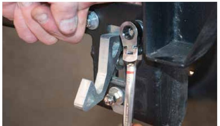
Shown to right are the additional bolts for the bump stop that can be adjusted for proper latching.
