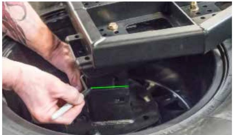
Flip arm over and position your tire mount into position. Tighten into place where you marked your lines.
