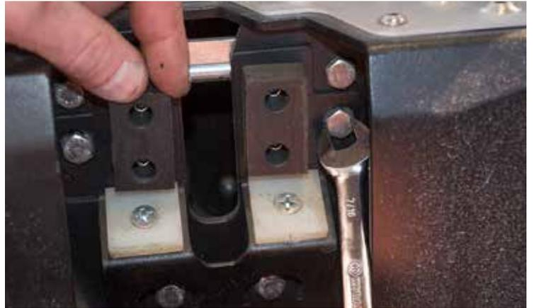
Using anti-seize provided, paste it around the threaded area of cap.
